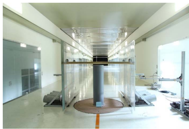
Figure A1 Installation of PVC cylinder
